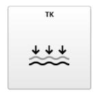
The amplification of very soft (G20) input sounds can be adjusted with the **[TK]** tuning tool. An increase of gain for very soft input sounds lowers the threshold knee point (TK) and vice versa.
